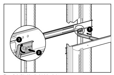
Figure 2-4. Attaching the latch bracket
